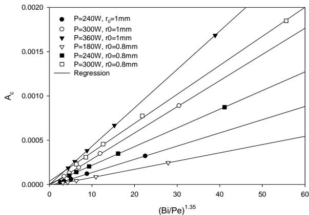
Fig. 10 Dimensionless cross sectional area vs.  $(Bi/Pe)^{1.35}$
