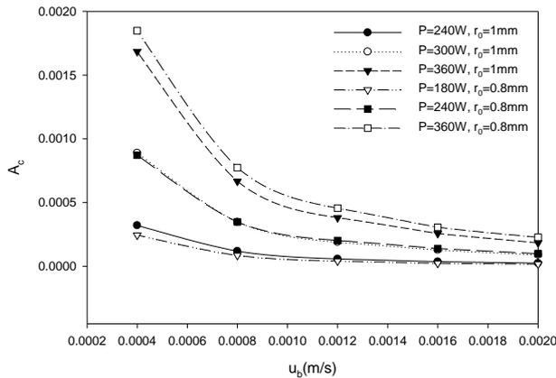
Fig. 9 Dimensionless cross sectional area vs. scanning velocity
