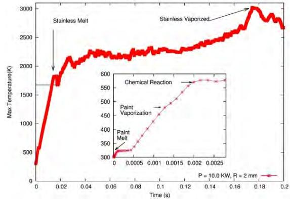
Figure 2 Variation of the maximum temperature during the laser irradiation for the case with laser power of 10 KW.
