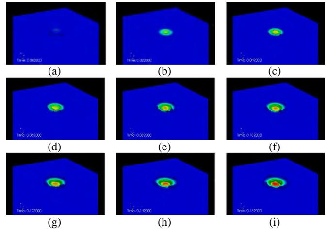
Figure 3 Solid and liquid phase during the laser irradiation Power =10 KW, R = 2 mm,  $I_{\text{max}} = 7.96 \times 10^4 \text{ W/cm}^2$  (Colored by temperature)
