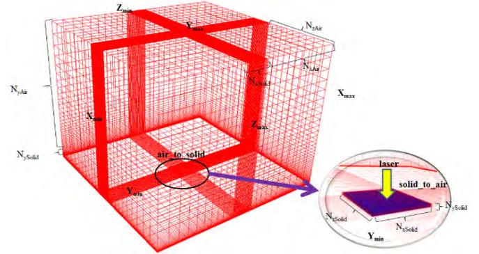
Figure 1 Illustration of computational domain
