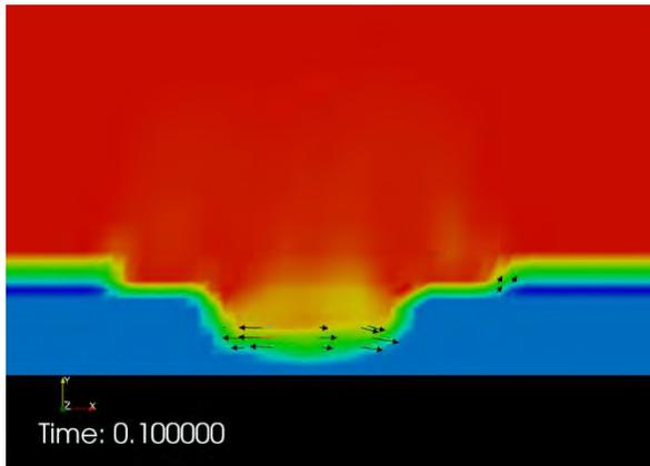
Figure 4 Marangoni force push on the interface between liquid and gas, the arrows indicate the direction of Marangoni force
