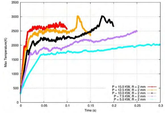
Figure 8 comparison of five cases with different laser power
