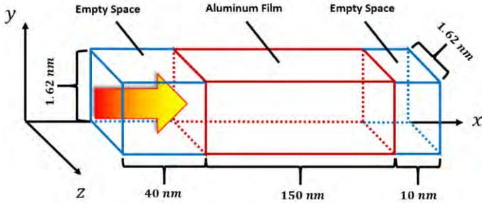
**Fig. 1 Schematic illustration of the modeled system.**
