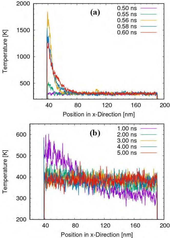
**Fig. 2 Temporal and spatial evolution of temperature. (a) The laser irradiation stage from 0.5 ns to 0.6 ns. (b) The stage after laser irradiation until 5 ns. (For the best interpretation of the calculated results, color version of this figure is seen online.)**
