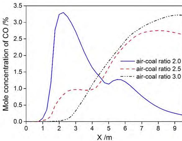
**Fig. 11** The curves of the CO concentration
