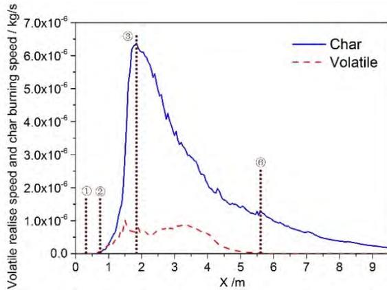
(a) Volatile release speed and char burning speed curve
