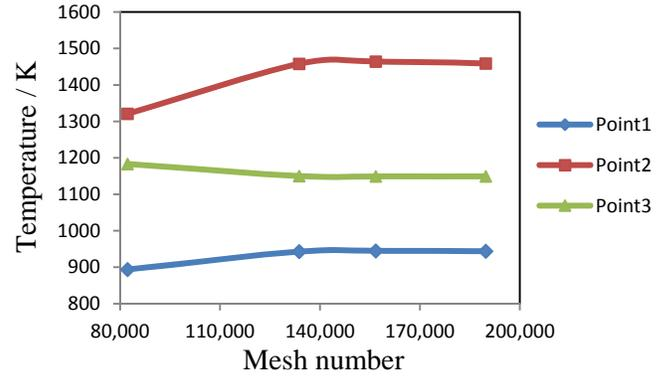
Fig. 3 Reference points temperature variation with the mesh number
