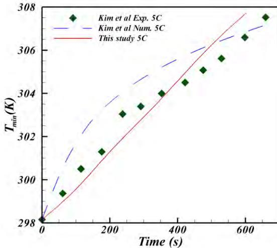
**Fig. 4 Comparison of minimum temperature inside the battery**
