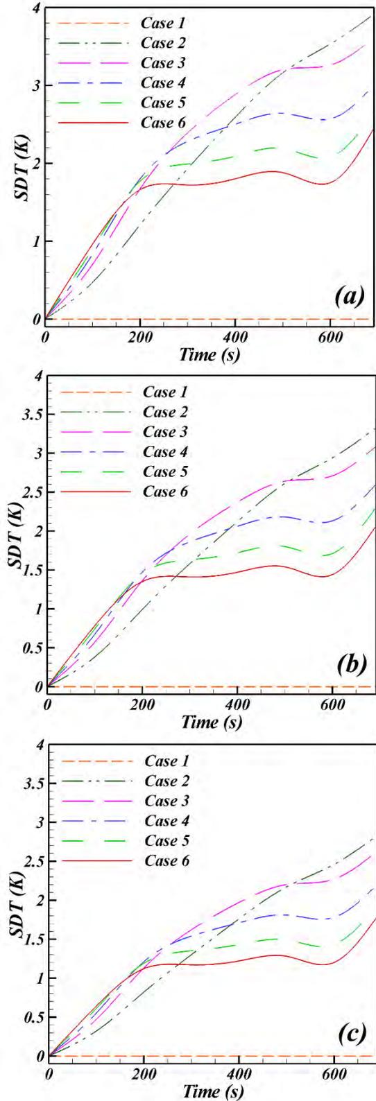
Fig. 6 SDT inside the battery cell versus time for inlet temperature of electrolyte flow of (a)  $288.15K$  (b)  $298.15K$  (c)  $308.15K$ , and inlet velocity of electrolyte flow of  $0.01 m/s$ .
