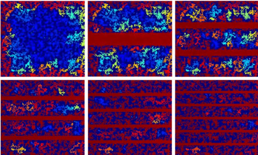
**Fig. 6** Electrolyte transport in cathode electrode after 500,000 timesteps.
