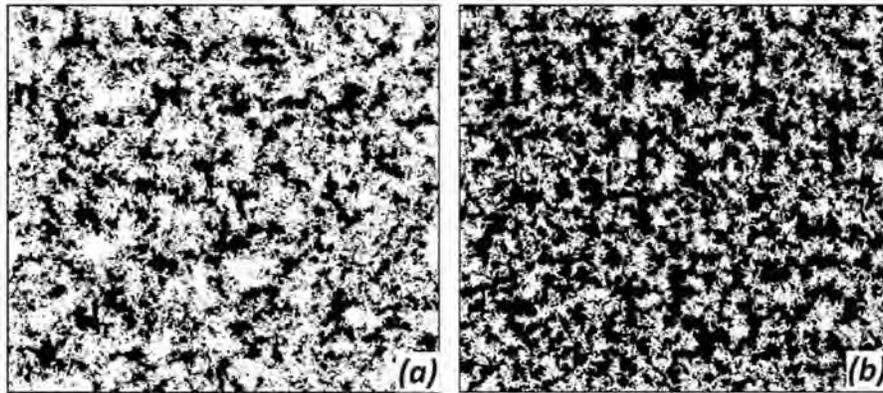
Fig. 1 Porous medium generation (a) Anode electrode  $p=0.6$  (b) Cathode electrode  $p=0.4$ .
