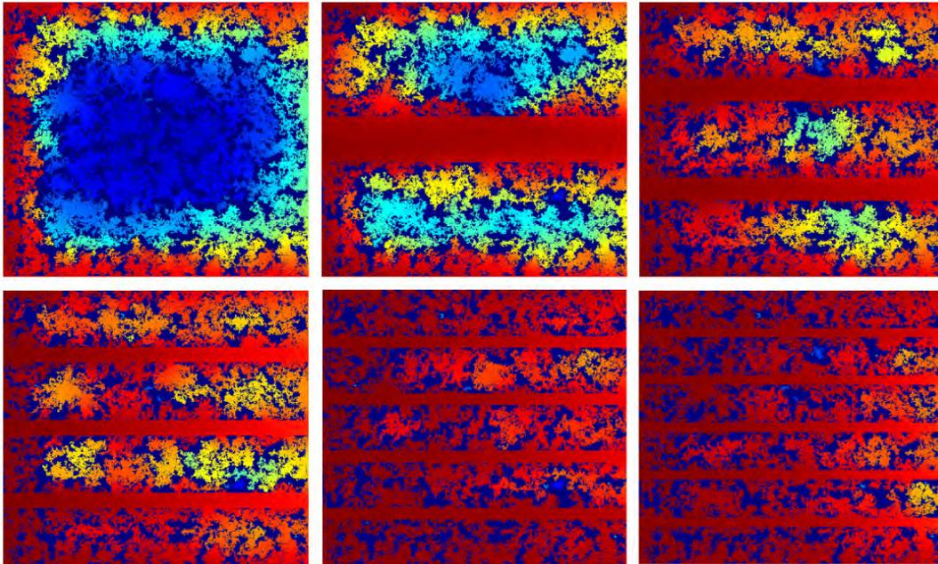
**Fig. 5** Electrolyte transport in anode electrode after 200,000 timesteps.
