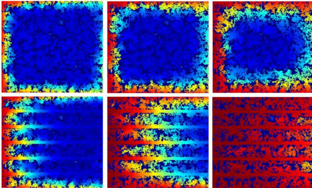
**Fig. 4** Electrolyte transport in anode electrode after 50,000 timesteps (Left), 100,000 timesteps (middle), and 200,000 (right) timesteps.
