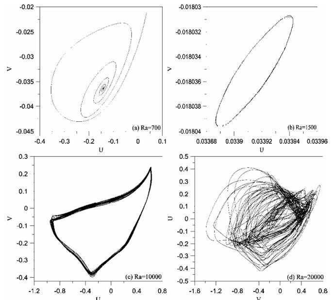
Figure 7 Velocity time trace at different Rayleigh numbers.
