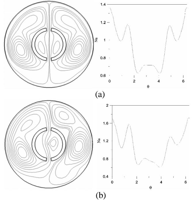
Figure 3 Steady streamline and temperature field for (a)  $Ra=700$  and (b)  $Ra=1000$ .
