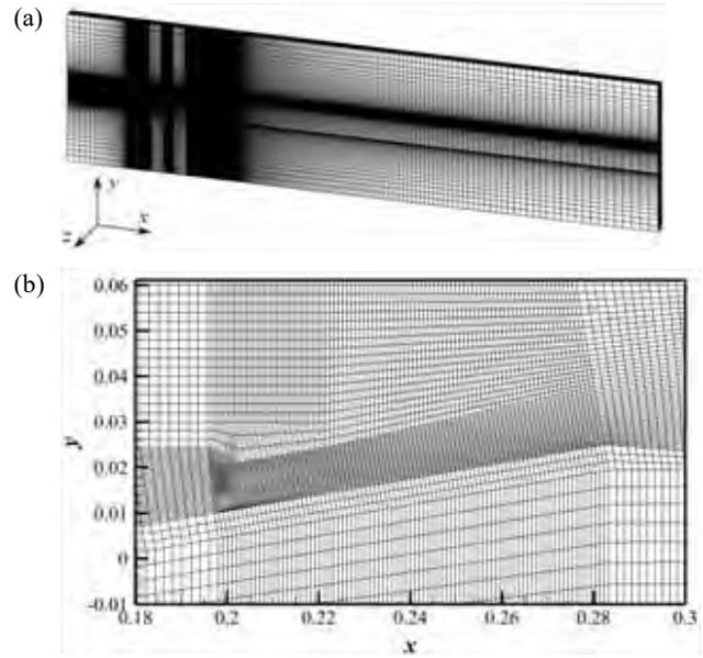
**Figure 4. Grid distribution. (a)The whole mesh; (b)Grid distribution of the cutback area in section  $xy$ .**
