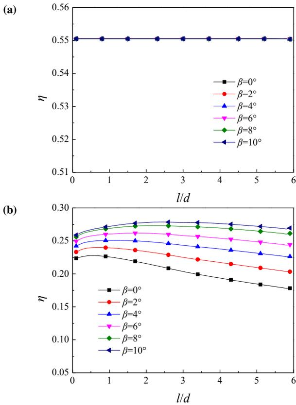
Figure 5.  $\eta$  along with the change of  $l/d$ . (a)Center line of slot downstream; (b)Center line of rib downstream.
