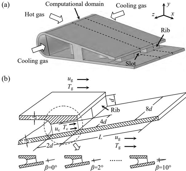
**Figure 2. (a) 3D model for trailing edge of turbine blade; (b) Schematic of trailing edge cutback.**
