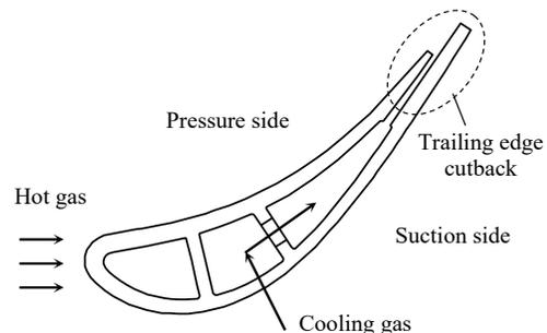
Figure 1. Schematic of turbine blade.
