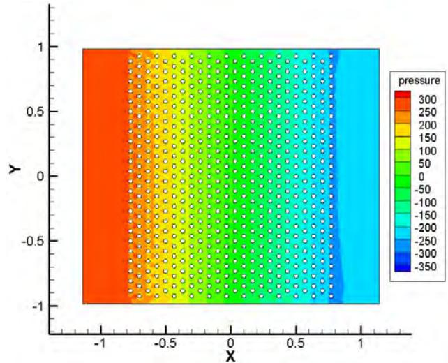
Fig. 16 Pressure field of 413K, 8m/s
