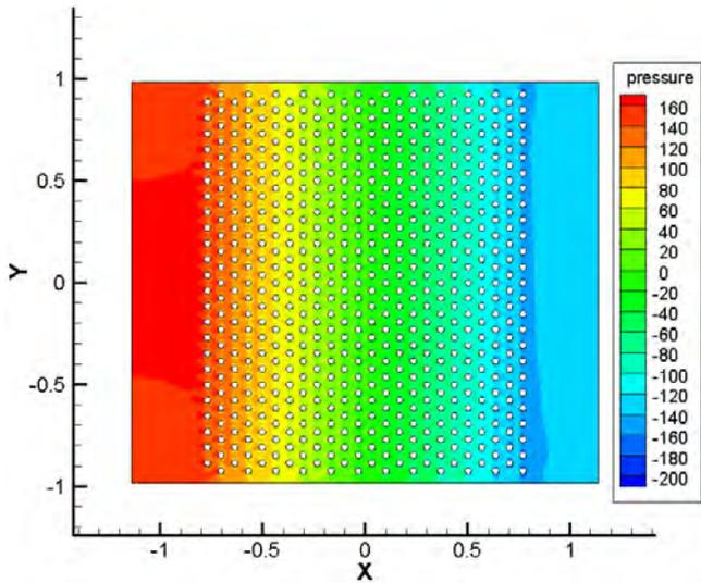
Fig. 13 Pressure field of 413K, 6m/s
