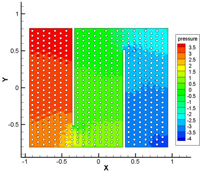
Fig. 22 Pressure field of 0.4m/s
