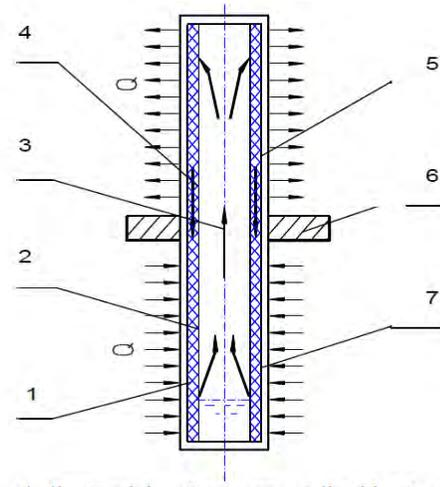
1- tube-shell, 2-wick, 3-vapour, 4-liquid, 5-condenser section, 6-clapboard, 7-evaporation section
