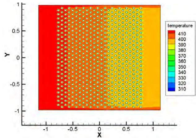
Fig. 11 Temperature field of 413K, 6m/s
