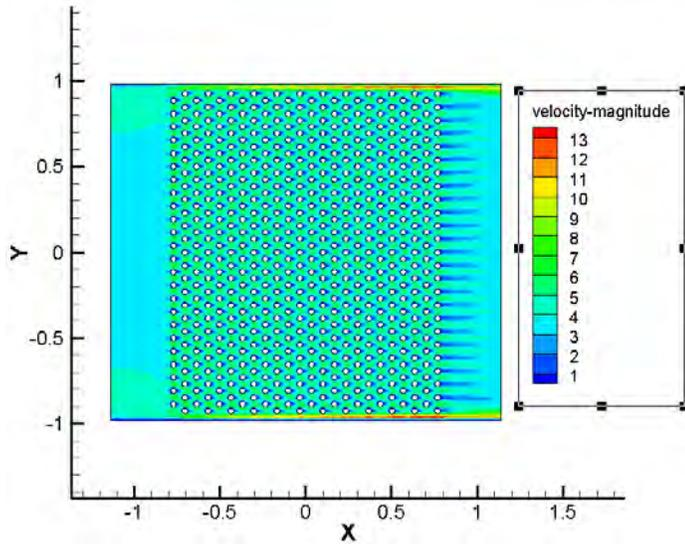
Fig. 9 Velocity field of 413K, 4m/s
