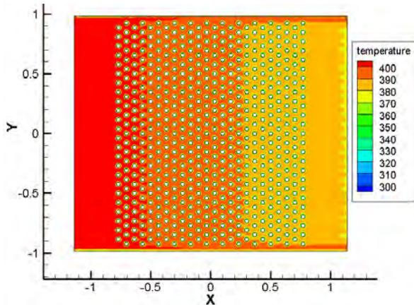
Fig. 14 Temperature field of 413K, 8m/s
