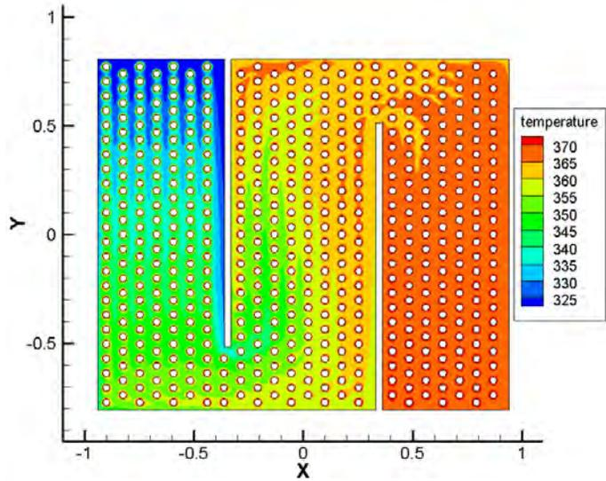
Fig. 17 Temperature field of 0.2m/s
