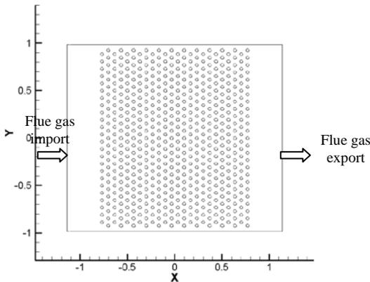
Fig. 6 physical model of flue gas side
