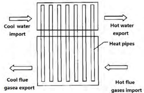
Fig. 2 Heat transfer model of heat pipe heat exchanger
