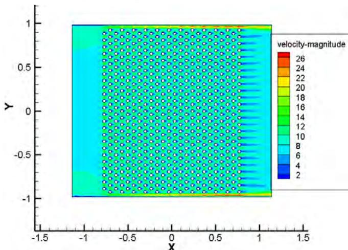
Fig. 15 Velocity field of 413K, 8m/s
