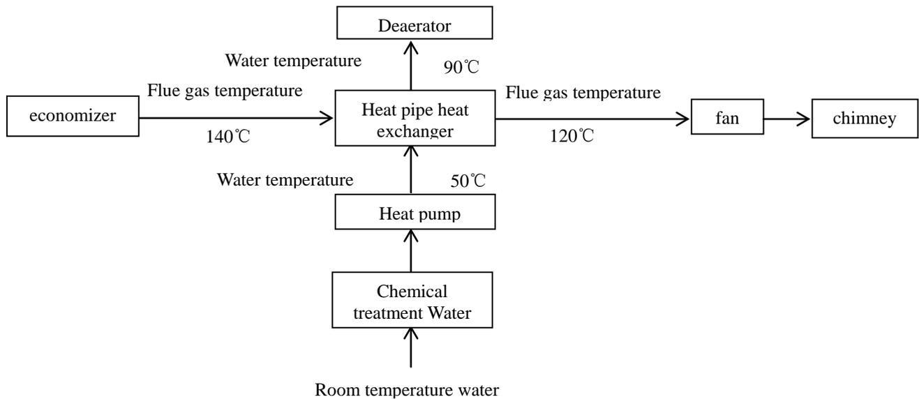
Fig. 5 Process flow diagram of the system of reclaiming residual heat of the flue gas with heat pipes
