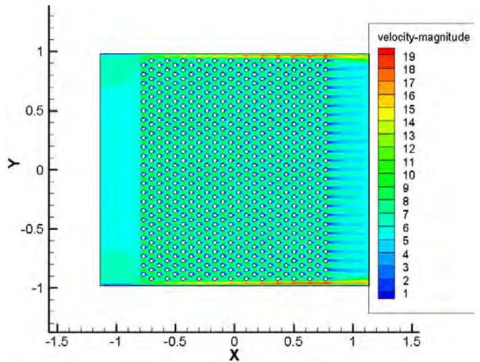
Fig. 12 Velocity field of 413K, 6m/s
