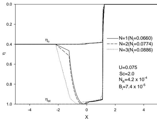
Fig. 6 Effects of numbers of existing sintered layers on the sintering process ( $\Delta=1.0$ ,  $U=0.075$ )
