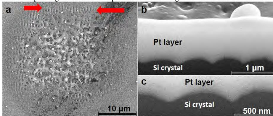
**Fig. 2.** (a) - LIPSS on the (100) surface of the silicon single crystal produced by two pulses at fluence 2.5-fold threshold of the single-pulse surface-modification. Red arrows show the location of the cross section produced by FIB to obtain SEM images of the sub-surface layer (b and c). Images (b) and (c) show no signatures of voids or fracturing, but show modified (amorphous) material on top of the ripples.
