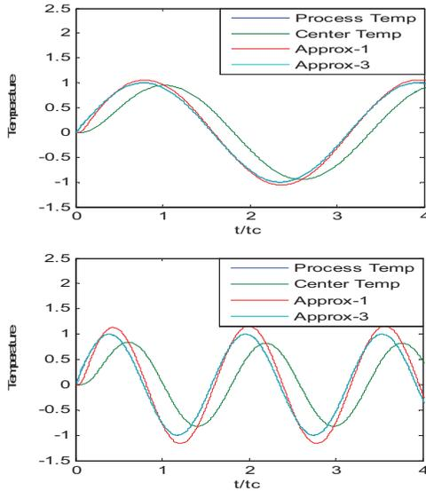
**Figure 5.** Dynamic compensation including up to third order time derivatives for  $Bi=4$ . (a)  $t_c \omega = 2$ , (b)  $t_c \omega = 4$ . Note that the curves corresponding to “Process Temp” and “Approx-3” overlap.
