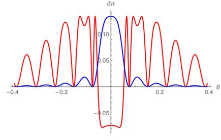
Fig. 8. Difference between classical and quantum detection error probabilities for a target with maximal (red) and small (blue) reflectivity.
