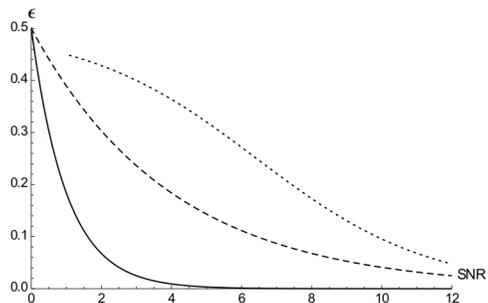
Fig. 1. Detection error probability upper bound  $\epsilon$  for  $M = 10^9$  entangled photon states ( $P_q$  - solid line), coherent unentangled photon states ( $P_l$  - dashed line), and a coherent integration of classical radar pulses ( $P_c$  - dotted line), with respect to the signal-to-noise ratio (SNR).
