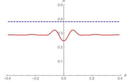
Fig. 9. Detection error probability for one quantum sensor fixed in the specular direction (blue) compared to the classical DEP (red) and the optimal quantum DEP (green).
