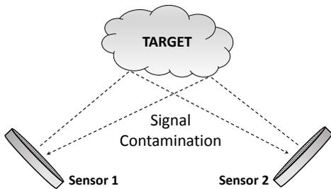
Fig. 2. A system composed of two sensors will increase the number of distinguishable modes. However, each sensor will generate photons that may be received as noise by the other. The result of this cross-contamination is an effective increase in the background noise experienced by each sensor and, consequently, the net background noise of the joint system.
