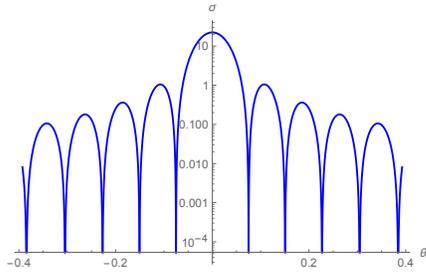
Fig. 5. Cross section of rectangular target near the specular direction.
