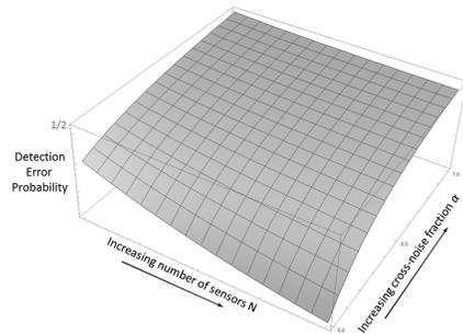
Fig. 3. The detection error probability of the system is reduced with increasing  $N$  and  $\alpha \ll 1$ . Conversely, as  $\alpha$  increases relative to  $N$  the detection error probability approaches the zero-information limit of 1/2.
