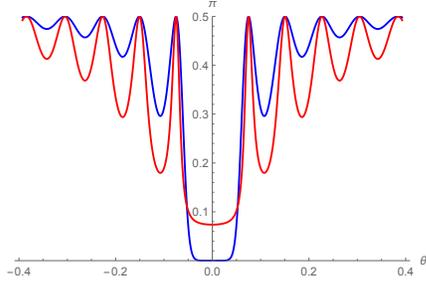
Fig. 6. Detection error probability for classical (blue) and quantum (red) sensing for a maximal reflectivity target.
