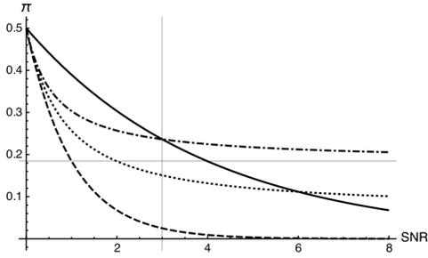
Fig. 4. Classical (solid line) and quantum detection error probability  $\pi$  as a function of the signal-to-noise ratio for  $\alpha = 0$  (dashed line),  $\alpha = 0.5$  (dotted line),  $\alpha = 1$  (dot-dashed line). Also shown is the asymptotic limit for the detection error probability with the maximal cross contamination  $\alpha = 1$  for arbitrarily large  $SNR$  (horizontal grid-line).
