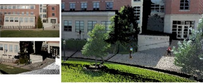
Fig. 3. Creating 3D planes for dynamic objects. Top Left : 2D video frame. Bottom Left : Video frame projected onto range scan without using our method for modeling moving objects. Right : 3D planes constructed for moving objects identified in video using our modeling method.
